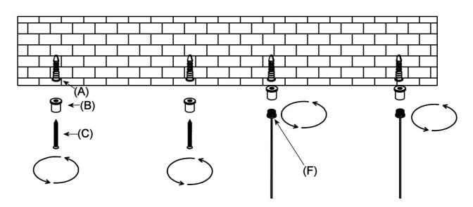
Using the fixing positions marked on your ceiling drill fixing holes taking care to avoid electrical supply cables. The unit is supplied with general purpose hardware for fitting the metal ceiling fittings (B) to a sound ceiling surface. Many situations require more specialist fittings, if you are in any doubt we recommend that you seek professional advice. The light should be fixed to a ceiling, joist or batten suitable to support the weight of the light fitting.
